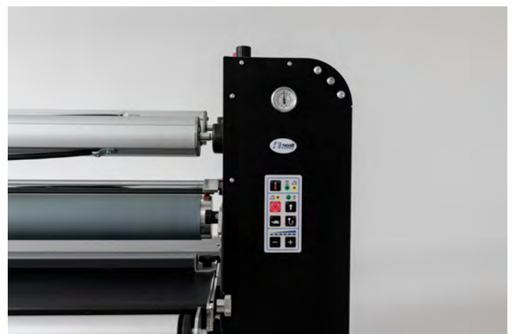
Interface and pneumatic control
